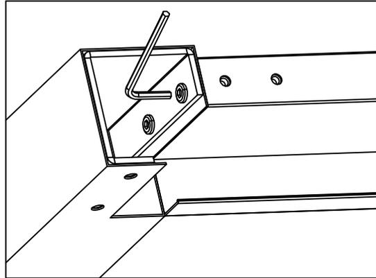
If there is any misalignment, adjust the concentricity of the holes, loosen the side bolts more than 10mm, and adjust the concentricity of the top threaded holes.
