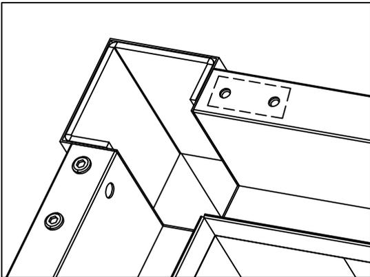
Assemble the lock top screw, and then tighten the side screws.
