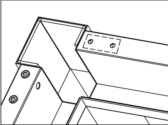
Check the top two threaded holes for misalignment.
