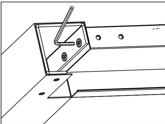
If there is any misalignment, adjust the concentricity of the holes, loosen the side bolts more than 10mm, and adjust the concentricity of the bottom threaded holes.
